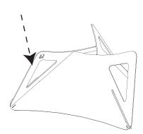
Pull the fin upwards and in direction of slot whilst applying downward force along the top edge. The side will easily pull away.
